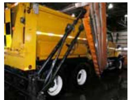
The box and wing attachments on this truck were fabricated by SGEU members in their welding fabricating shop in Regina, SK.
